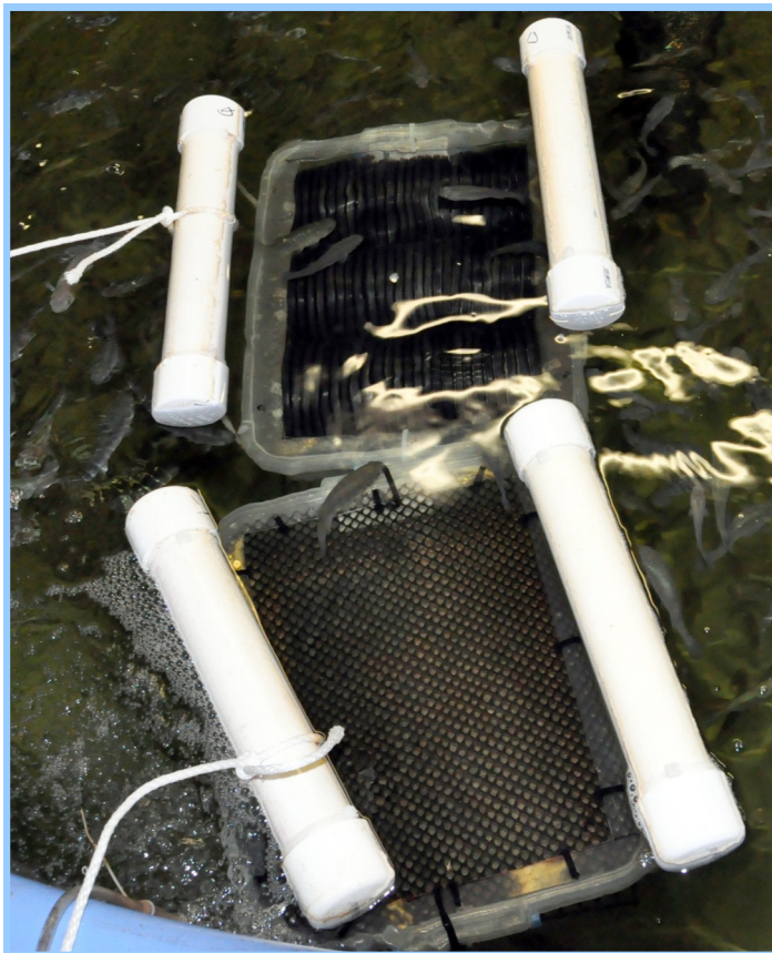
Different egg collector designs deployed for spawning substrate selection trials. Capped PVC tubes act as floats and the harnesses they are attached to maintain collectors at a shallow depth below the surface.
